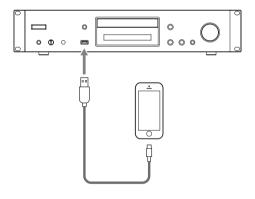
• Connect an iPod to the iPod/iPhone USB connector on the front of the unit.
