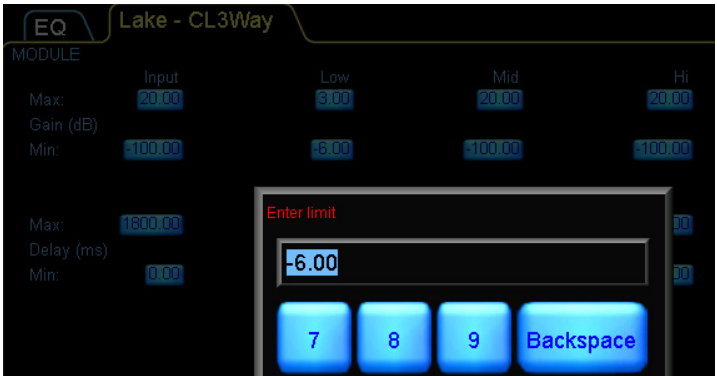
Figure 19-8: Restricting the Minimum Gain Value for Output 1
