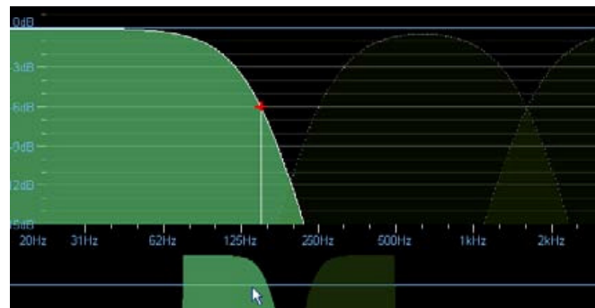
Figure 4-47: Splitting and moving the low channel HPF
