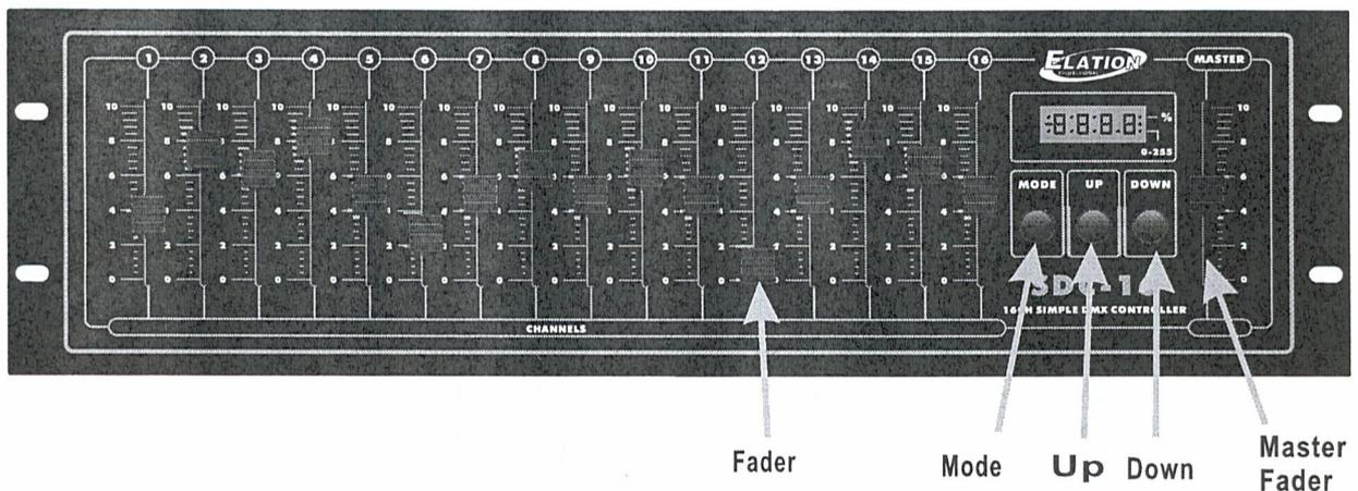
1. When switching on the power supply, the LED window will display the start DMX channel address. It can be "A001". If there are no character and number display, check the power whether it's correctly connected.
