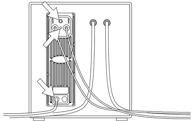
Connect the subwoofer to the mains power supply using the cable provided. Connect the appropriate end of the cable to the POWER socket on the back connection panel of the K3st SUB. Connect the other end to the main power supply.
