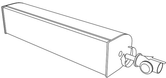
Take a K3st TOP and screw the stand adapter in the nut placed in the bottom of the cabinet. Repeat with the other top and adapter.
