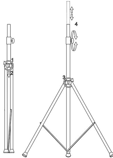
Take the floor stands, fully spread out the legs loosening the locking screw (1), pulling out the legs (2) and retightening the locking screw (3). Adjust stand height according your wish (4). Place the floor stands where desired, be sure they are stable and safe.
