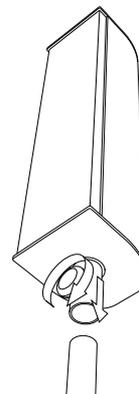
Place each K3st TOP on its stand and tighten the locking screw on the adapter.
