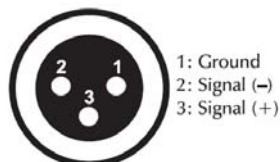
DMX-output XLR mounting-socket:
