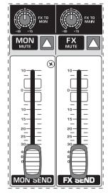
Fig. 2.6: Aux send controls of the main section
