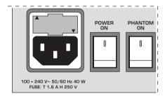
Fig. 2.17: Voltage supply and fuse
