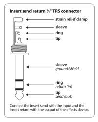
Fig. 4.5: Insert send return  $\frac{1}{4}$ " TRS connector
