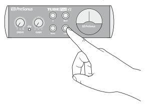
5. Speak into the microphone while watching the VU meter on the front panel and slowly turning the TubePre V2 Gain knob clockwise.
