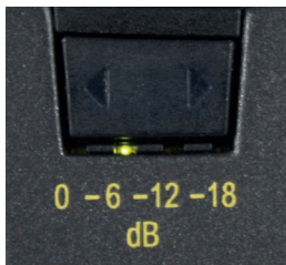
Figure 2: Preattenuation Pad
