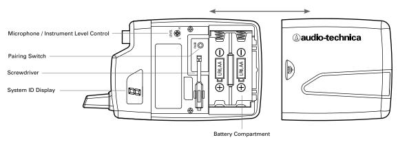
Figure C — ATW-T1001 UniPak® Transmitter
