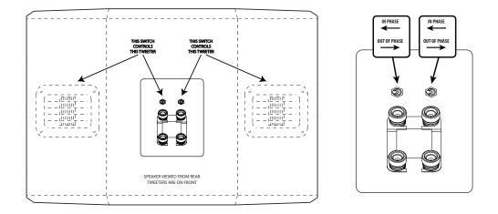
The Airmotiv E2 will provide the most precise sound imaging and localization when configured as a conventional direct firing or "bipole" surround speaker, and this is what most modern surround sound standards recommend. To configure the Airmotiv E2 for this mode, simply set both switches on each Airmotiv E2 to IN-PHASE.
