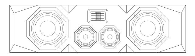
The Airmotiv C2 is a three way center channel loudspeaker, featuring a 32mm Airmotiv folded ribbon tweeter, dual 3" woven fiber midrange drivers, and dual 6" woven fiber woofers. The Airmotiv C2 is designed to be used as a center channel speaker in high end home theater installations.
