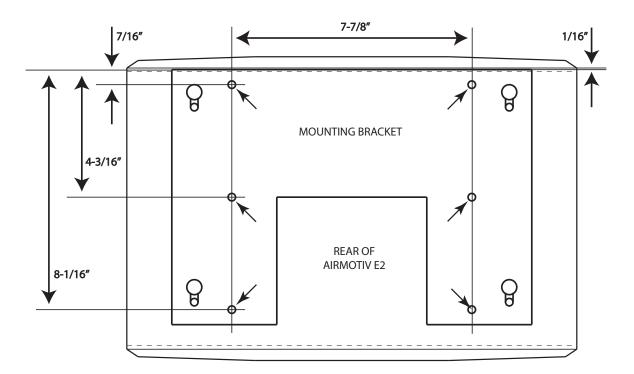
Note six (6) wall bracket mounting holes.
