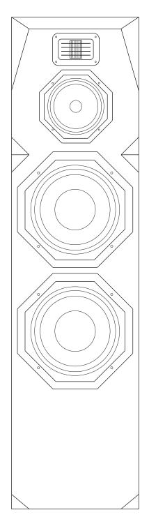
The Airmotiv T2 is a three way, floor standing, tower loudspeaker, featuring a 32mm Airmotiv folded ribbon tweeter, a 5-1/4" woven fiber midrange, and dual 8" woven fiber woofers. The Airmotiv T2 can be used in an audiophile stereo setup, or as a main front speaker in a home theater installation, or you could use a full set of Airmotiv T2's as the basis of a really high end home theater installation.
