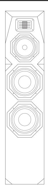
The Airmotiv T1 is a three way, floor standing, tower loudspeaker, featuring a 32mm Airmotiv folded ribbon tweeter, a 5-1/4" woven fiber midrange, and dual 6" woven fiber woofers. The Airmotiv T1 can be used in an audiophile stereo setup, or as a main front speaker in a home theater installation, or you could use Airmotiv T1's "all around" in a high end home theater installation.
