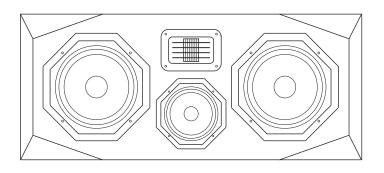
The Airmotiv C1 is a three way center channel loudspeaker, featuring a 32mm Airmotiv folded ribbon tweeter, a 3" woven fiber midrange, and dual 5-1/4" woven fiber woofers. The Airmotiv C1 is designed to be used as a center channel speaker in high end home theater installations.
