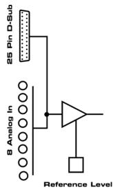
One of the main issues when working with an AD-converter is to maintain the full dynamic range within the best operating level. Therefore the M-32 AD internally uses hi-quality electronic switches, which introduce no additional noise or distortion to the audio path. The key ANALOG INPUT allows for a perfect adaptation of all 32 channels to the most often used studio levels.
