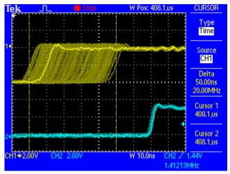
The cleaned and jitter-freed signal can be used as reference clock for any application, without any problem. The signal processed by SteadyClock is of course not only used internally, but also available at the units word clock output. It is also used to clock the digital outputs MADI and ADAT.
