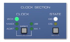
A selection of DS and QS is also possible when using external clock (Slave). If the M-32 AD should operate at 192 kHz, but receives a synchronous word clock of 48 kHz, the button STATE activates DS or QS mode. This way, AD-conversion and digital outputs are configured to operate in the frequency ranges Single Speed, Double Speed or Quad Speed.
