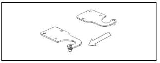
13.Put the hinge pin in the hole of the fridge door and tight the screws of the hinge. Put them in point 1 removed device cover on again, tight the screws and clip the cover caps on.
