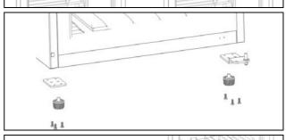
10.Unscrew the hinge pin and insert it to the other side of the door hinge. Screw the foot bracket and door hinge each at the opposite sides and screw the feet on again.
