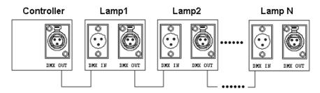
The shield connection is pin 1, while pin 2 is Data Negative (S-) and pin 3 is Data positive
