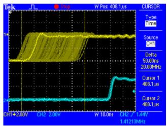
The cleaned and jitter-freed signal can be used as reference clock for any application, without any problem. The signal processed by SteadyClock is of course not only used internally, but also available at the ADI-642's word clock output. It is also used to clock the digital outputs MADI and AES/EBU.
