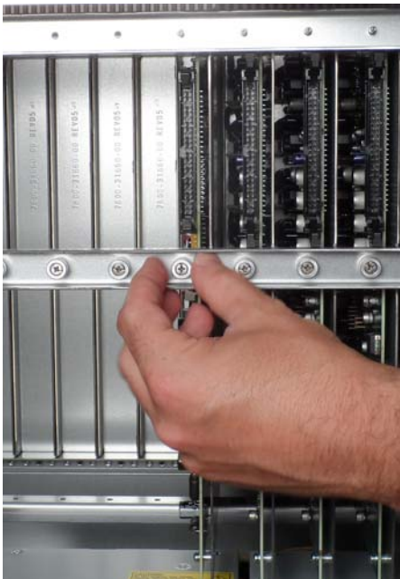
Figure 7. Securing the card to the Stage 64 chassis
