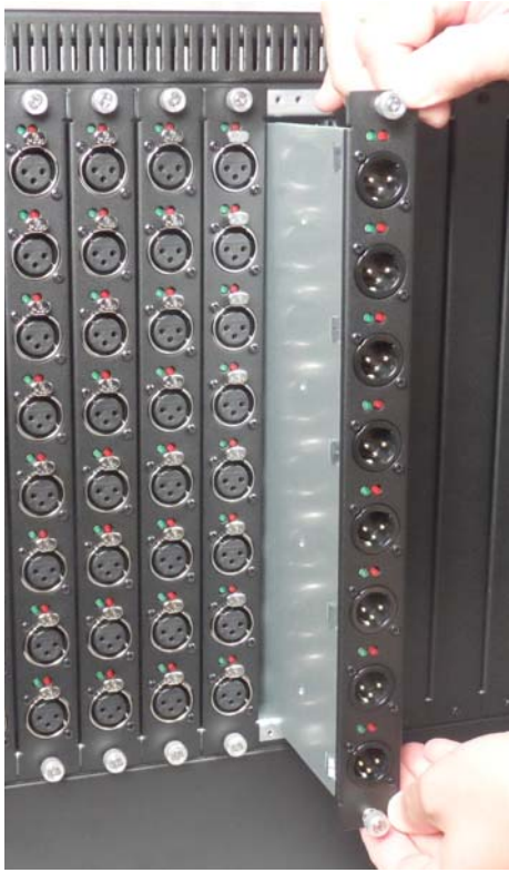
Figure 4. Sliding the card into the Stage 64 (SRO card shown)
